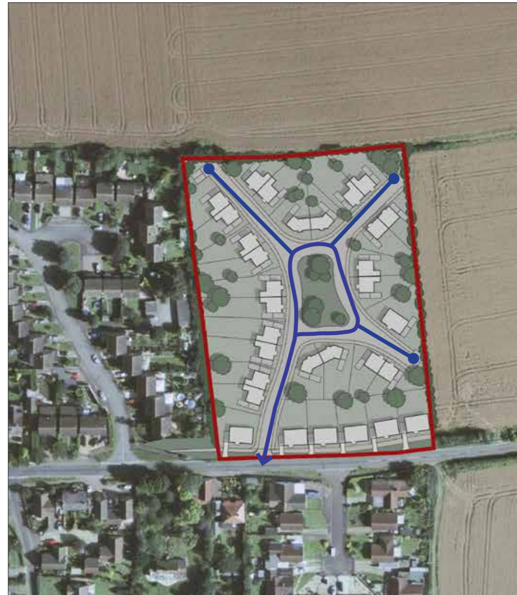
Fig 4.2. Diagram showing the route through Development Site 1 considering the possibility of locating the existing electric powerline underground.
