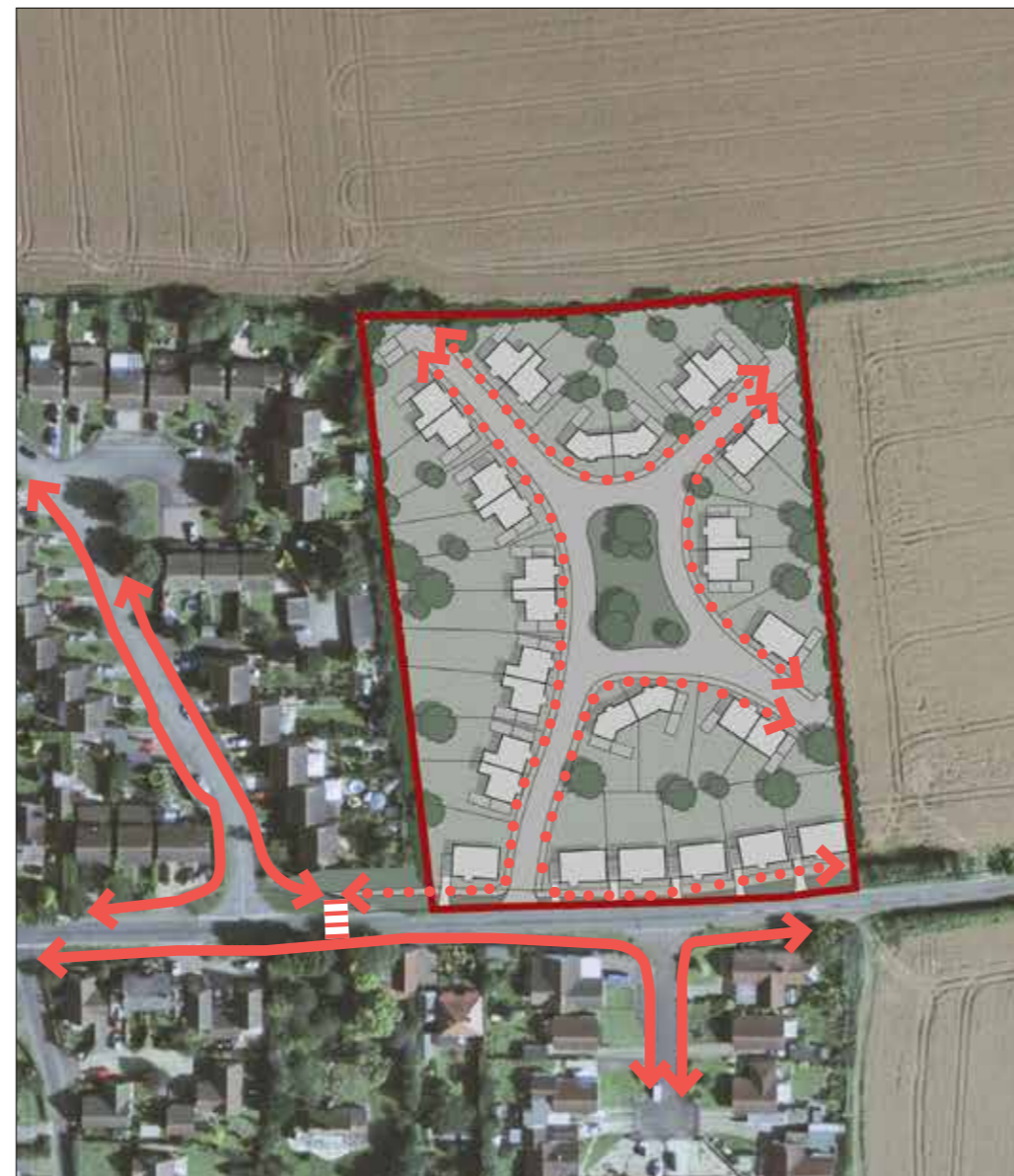
Fig 4.6. Diagram showing the existing and proposed footways through Development Site 1 and the surrounding areas. It illustrates a potential pedestrian crossing to improve existing and future connections.
