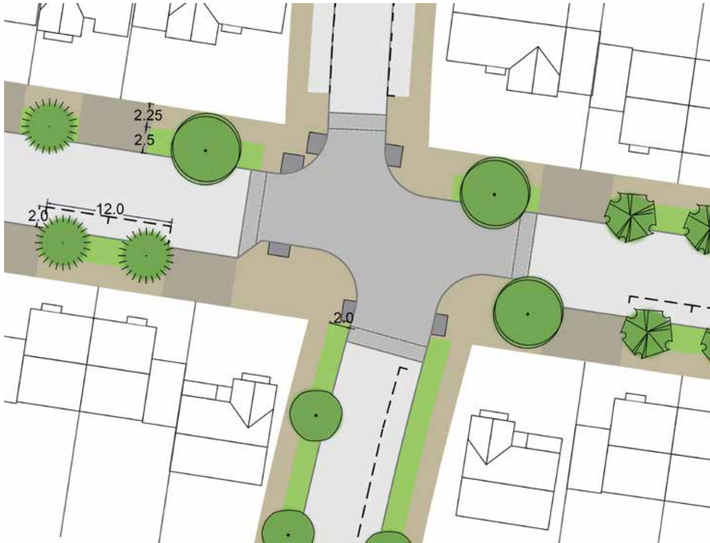
Figure 80: Diagram showing a typical neighbourhood junction with trees and their relationship with properties, parking spaces as well as tree-pit and verge sizes (dimensions shown given in metres). These dimensions are considered best practice but not all locations will have ideal conditions, thus a discussion with the Local Authority and highways team should be carried out to find the best balance to ensure the street function and the longevity of trees.
