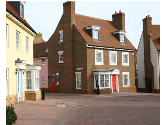
Shared surfacing can identify a change in direction or emphasise key spaces
