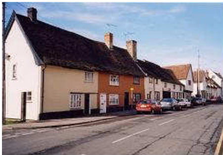
Bargeboards, overhangs, large chimneys, one-and-a-half storeys with dormers, strong colours for highlighting timbers
