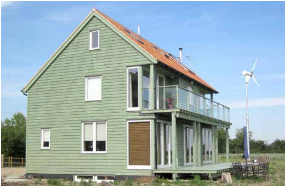
Example of contemporary architecture in Birdbrook. Sustainable house constructed to Passivhaus standards. Designed to be self-sufficient with a wind turbine, rainwater collection, reed-beds for sewage treatment and natural ventilation. RIBA East Building of the Year 2011. Photo courtesy of Modece. Source: http://www.modece.com
