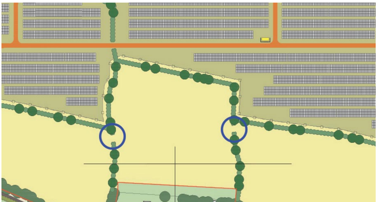
Amendment E - Gaps introduced to hedgerows to provide access between fields for agricultural purposes.
